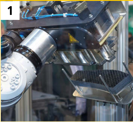
Step 1: A robot picks up the thermoplastic composite sheets and warms these in the gripper.
