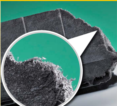
Foaming glass-fibre reinforced plastics: with ProFoam without additional shearing.
