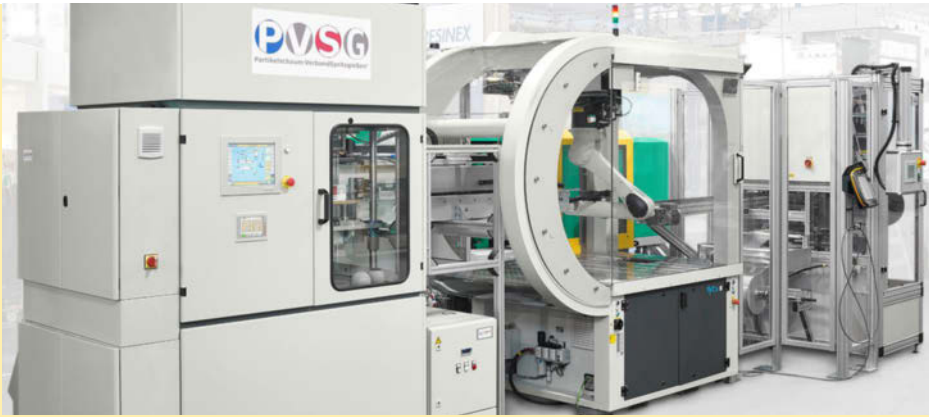
Compact production cell: Six-axis robotic system links foaming system and ALLROUNDER.
